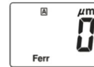
2. **Press the sensing tip of the probe** to contact **Standard Coating plate 102 $\mu\text{m}$** , coated surface tightly. Wait for the reading to appear and measurement is completed (one “Beep” sound announced), then you can move the Gauge away. Press “CAL” button **over 3 sec** to enter calibration mode. LCD will display “CAL” **blinking**.
