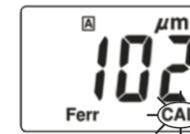
3. In calibration mode, use ▲ or ▼ button to adjust readings until it matches the standard's thickness (102  $\mu\text{m}$ ).
