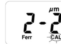
4. Place the standard thickness foil with the standard thickness of 102 microns on the uncoated calibration disc.
