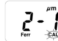
3. Place the sensor of the unit straight on the disc until a **beep sounds twice** and on the display appears “2-2”. (The device automatically calibrates to the uncoated area).
