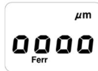
The **factory setting is sufficient** to precisely **determine differences** in the paint thickness on the vehicle.
