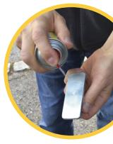
**1. Before use, degrease** the supplied adapters with silicone remover or brake cleaner.
