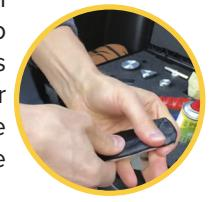
**3. Degrease the painted surface to be treated** (with silicone remover or brake cleaner), it must be **free of grease, clean and dry** before treatment.
